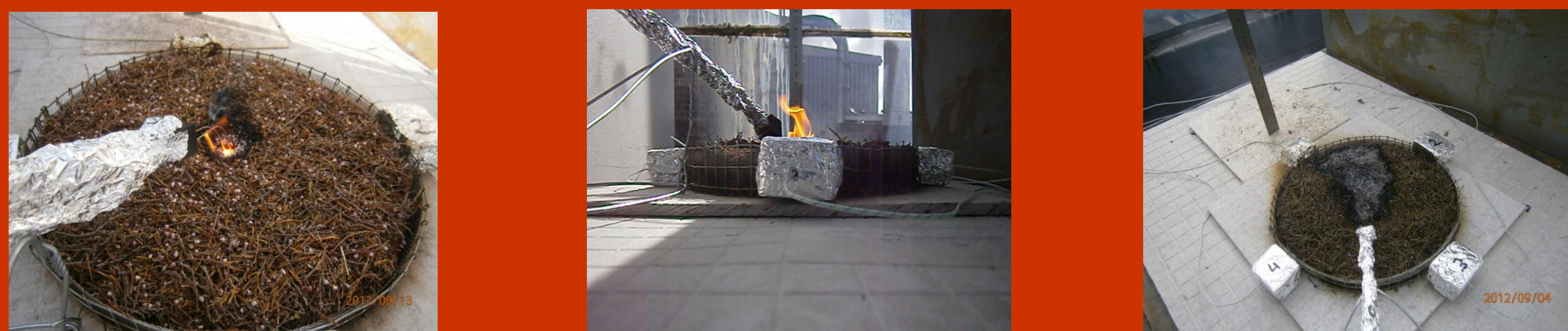
Figure 1. Experimental tests performed in the laboratory to assess the flammability properties of peat/litter fuel beds.
